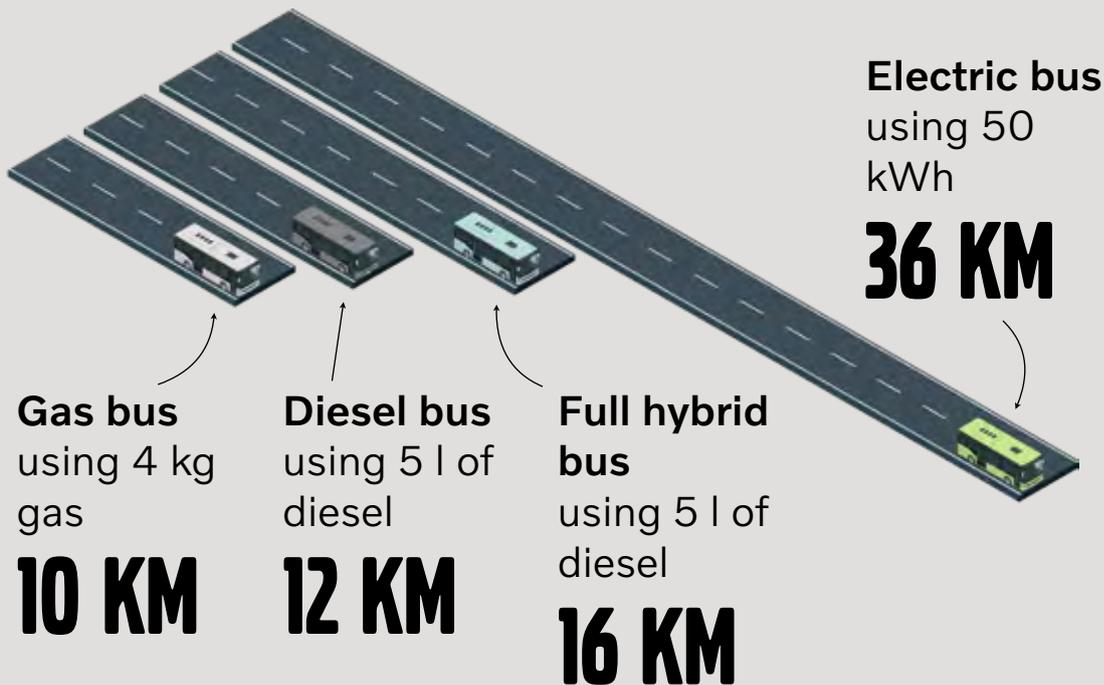
The calculation is based on tank-to-wheel energy consumption. Energy value of different types of fuel has been converted to kWh, where 4kg CNG = 5l diesel = 50 kWh electricity. Conventional diesel is used as a benchmark (100%) to compare results.
